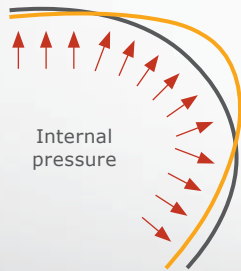
Non-flat carcass line design
