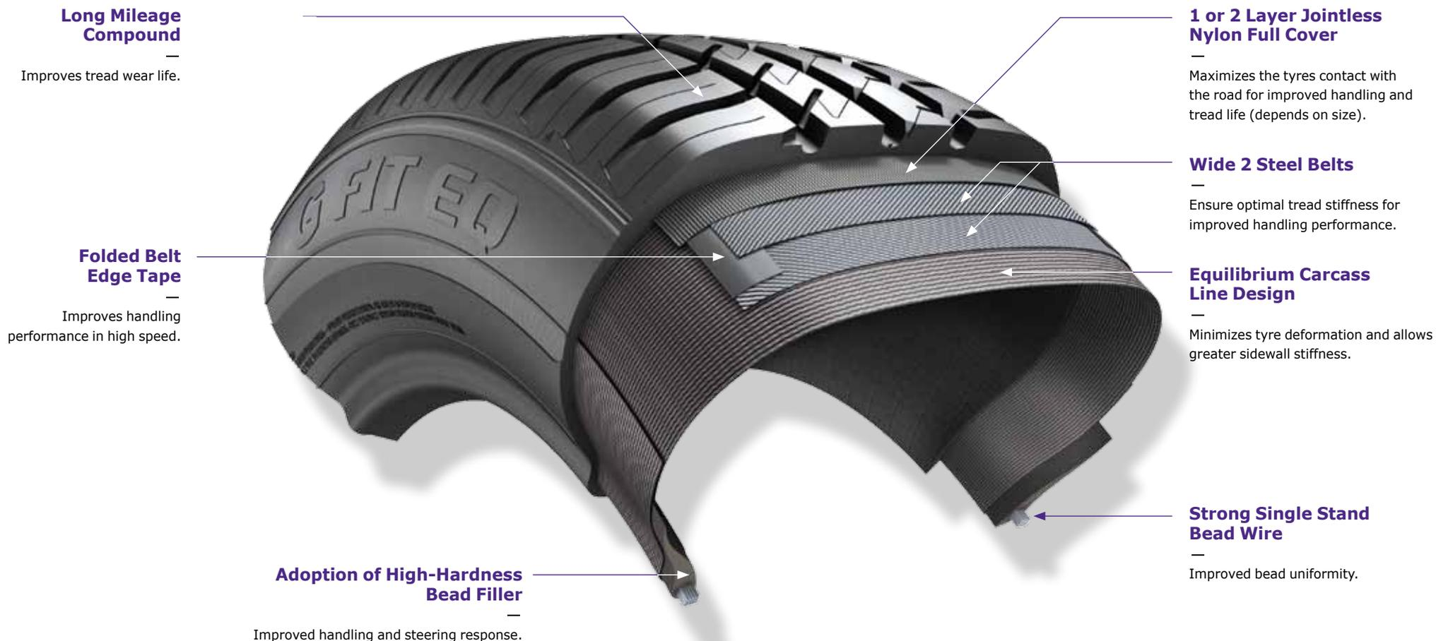
\* The model size in the structural diagram is for the 195/65R15H tyre, and the descriptions of structural diagrams may vary by size.
